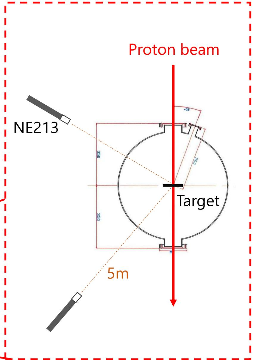
In advance of the experiment at FFAG, **detector test** was conducted to check the response and detection efficiency at FRS, JAEA.
