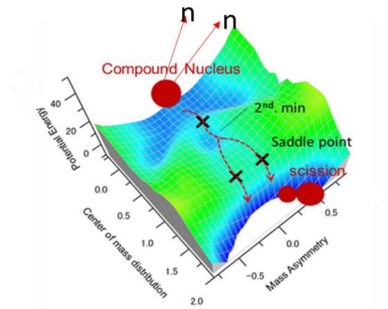
Figure 1 It is a diagram that considers only neutron emission from the compound nucleus, and is a diagram in which a fission path is projected on the potential energy surface. The saddle points are marked by the symbol “+”.
