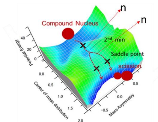
Figure 1 It is a diagram that considers neutron emission in all the processes of fission, and is a diagram in which a fission path is projected on the potential energy surface. The saddle points are marked by the symbol “+”.
