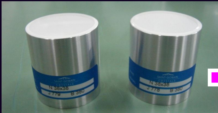
Saint-Gobain BrillLanCe380 Size: \phi 38 \times 38 \text{ mm}^3
