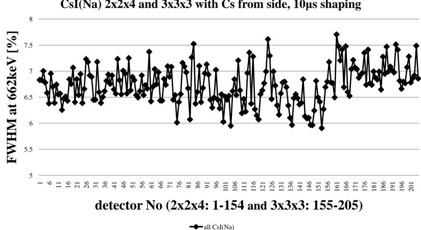
CsI(Na) 2x2x4 and 3x3x3 with Cs from side, 10µs shaping
