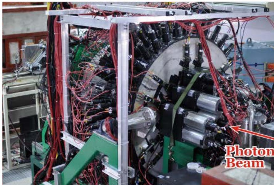
Target: 45 mm thick LH<sub>2</sub> & LD<sub>2</sub>
