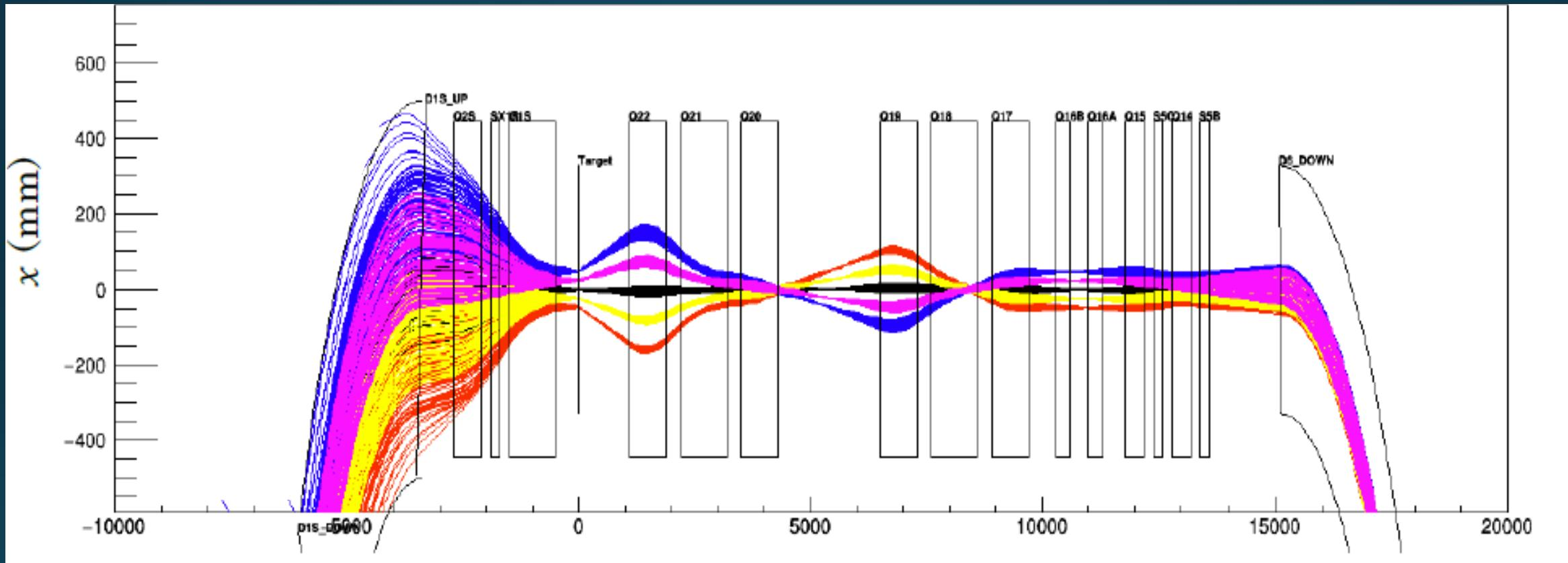
Beam momentum spread -> Position spread on target
