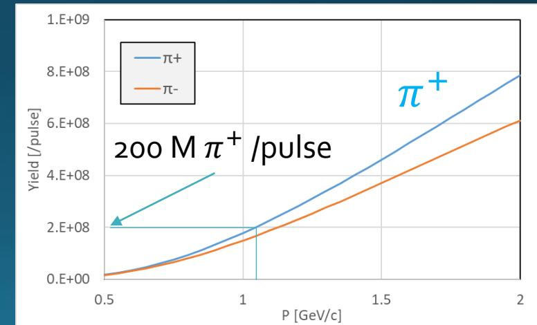
3deg. Ext. angle,  $5.0 \times 10^{13}$  ppp on 50% loss target
