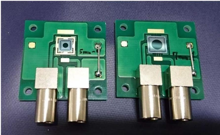
Fig. 2 Photograph of prototype neutron fluence monitors based on the SiPDs with the thickness of 320  $\mu\text{m}$  and the size of 5 x 5  $\text{mm}^2$  and 7 x 7  $\text{mm}^2$ .
