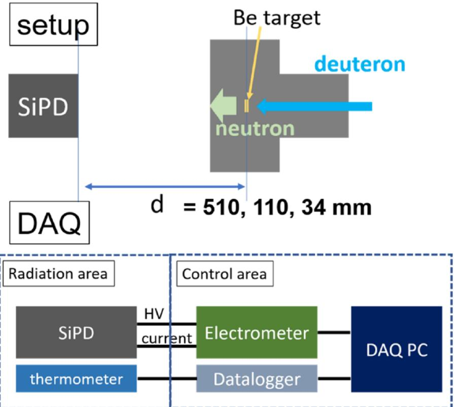
Fig. 4 Experimental setup. Leakage current of SiPD was measured changing distance ( $d$ ) between SiPD and Be target. Electrometer was used for applying bias voltage and measuring leakage current. Thermometer was also mounted near SiPD and the temperature was recorded with datalogger.
