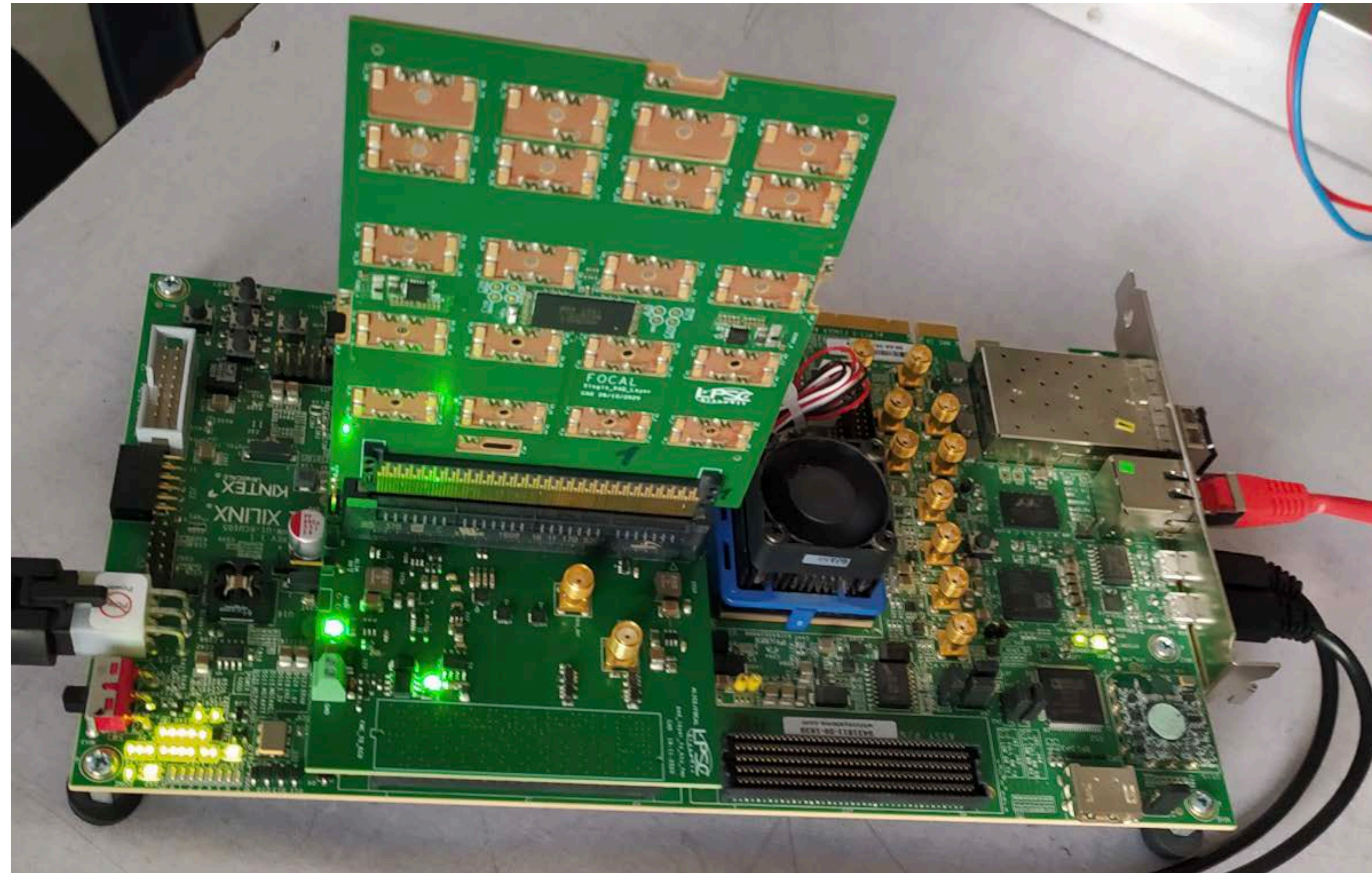
Grenoble LPSC: Single pad board connected to the KCU105 via the test interface board
