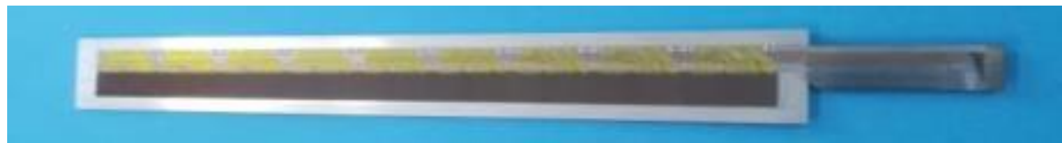
Developments with flex cables for medical application: proton-CT Bergen, Norway
