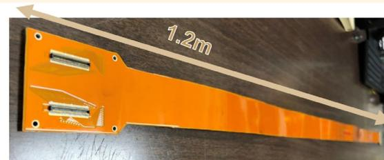
Long data bus extender developed in Japan
