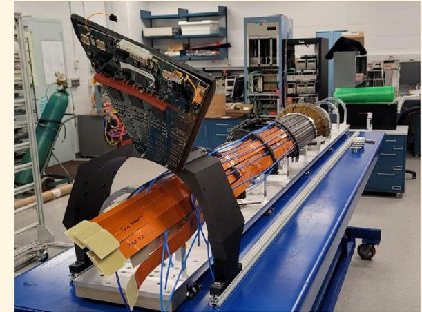
Barrel assembly test at BNL
