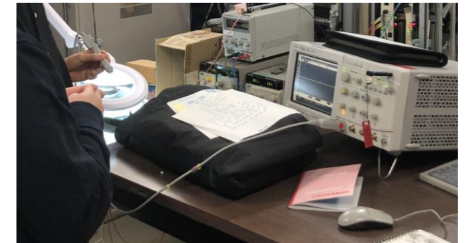
Measurement of output signal using oscilloscope
