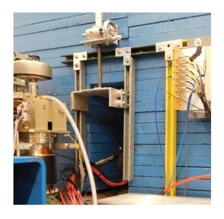
Limit of the detector size is related with the Pb (blue) whole and how far the ZDC (in the Pb hole) can be moved backward.
