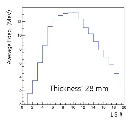
If the tungsten is too thick, more particles are absorbed in the tungsten, thereby relatively smaller energy deposit behind.
