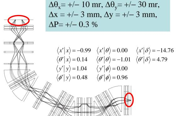
In the dispersion matched mode, trajectories at F3 and before the target are measured.
