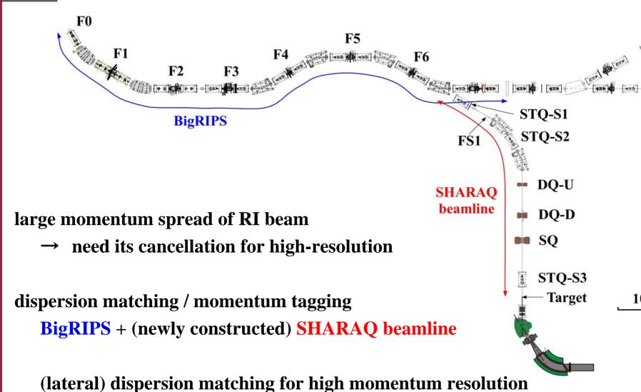
(lateral) dispersion matching for high momentum resolution angular dispersion matching for high angular resolution
