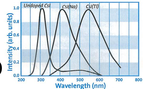
Figure 1. Scintillation emission spectrum of CsI
