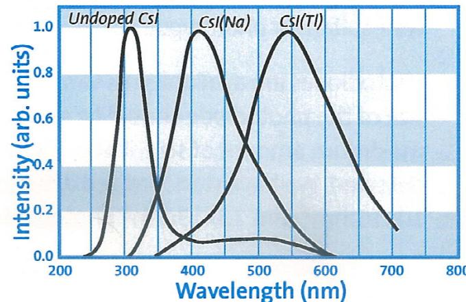
Figure 1. Scintillation emission spectrum of CsI
