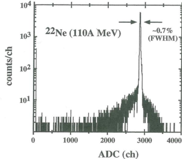
Fig. 1. Pulse height spectrum of the NaI(Tl) detector for  $^{22}\text{Ne}$  beam of 110A MeV.
