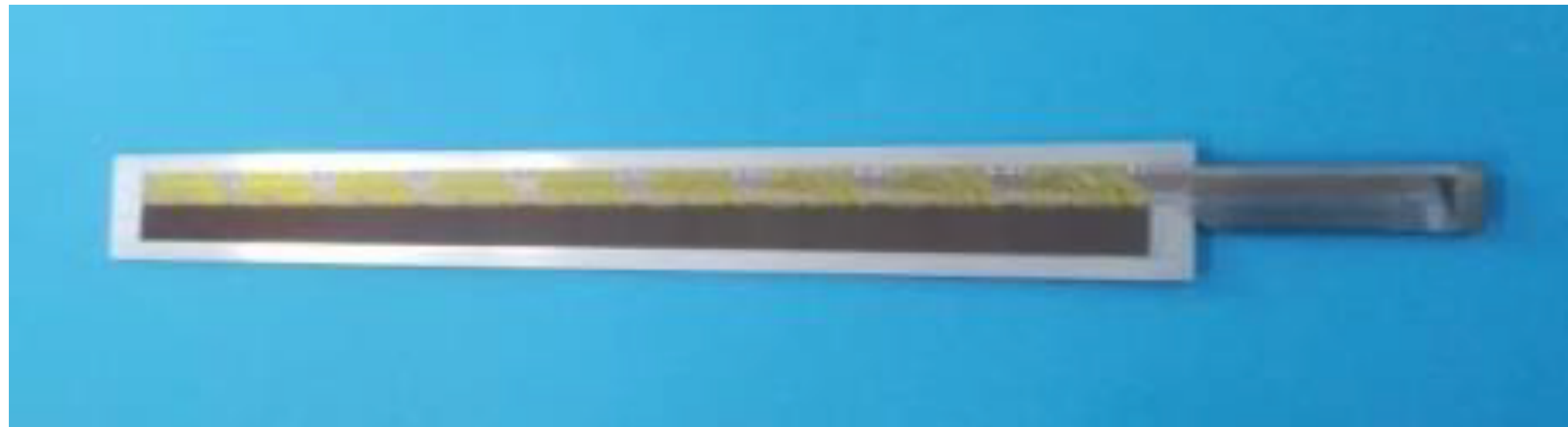
9 ALPIDE chips on a flex cable: 30 x 1.5 cm 2 (developed for pCT application )
