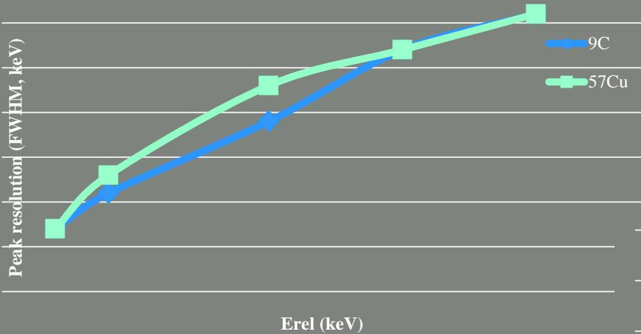
9C Breakup Resolution w Pb target 50mg/cm<sup>2</sup>
