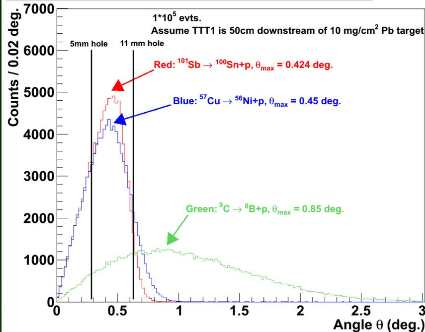
Detection Efficiency, TTT1 at 50cm, TTT2 at 80cm, with 5mm circular hole
