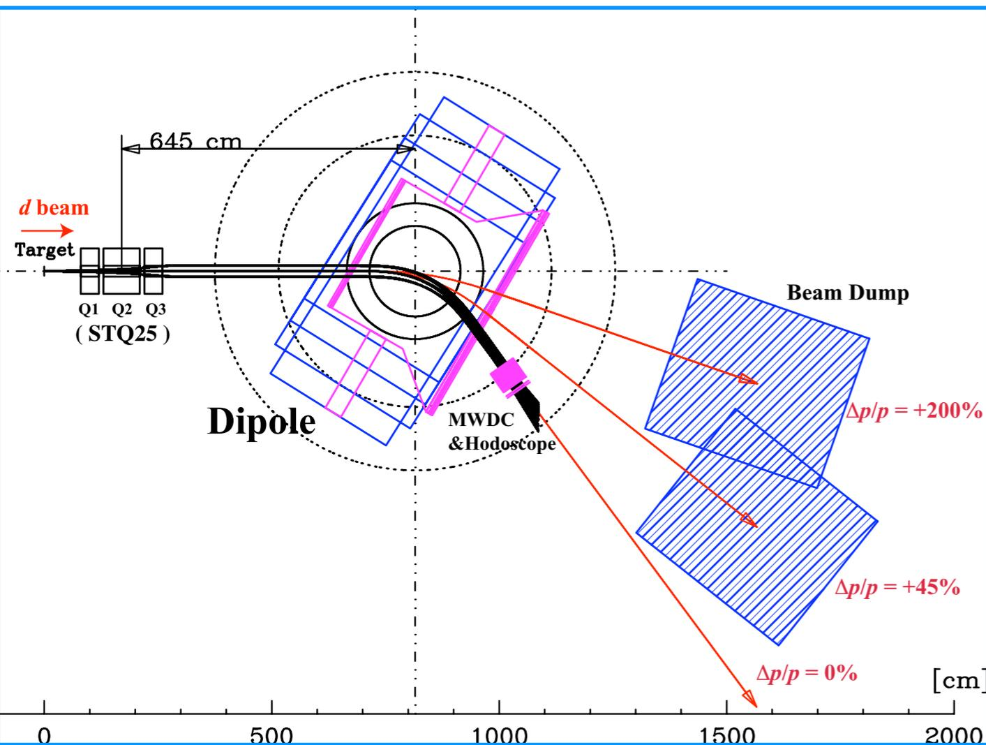
In experiments with polarized deuteron beams **high momentum resolution**  $p/\Delta p \sim 1600$  for 1.5 GeV/c proton
