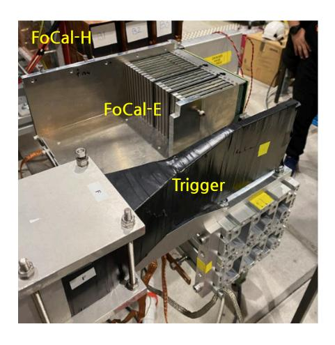
Prototype of the ALICE FoCal (FoCal-E + H) was installed at the SPS beam line and measured positrons and charged pions from September 15 to 21.
