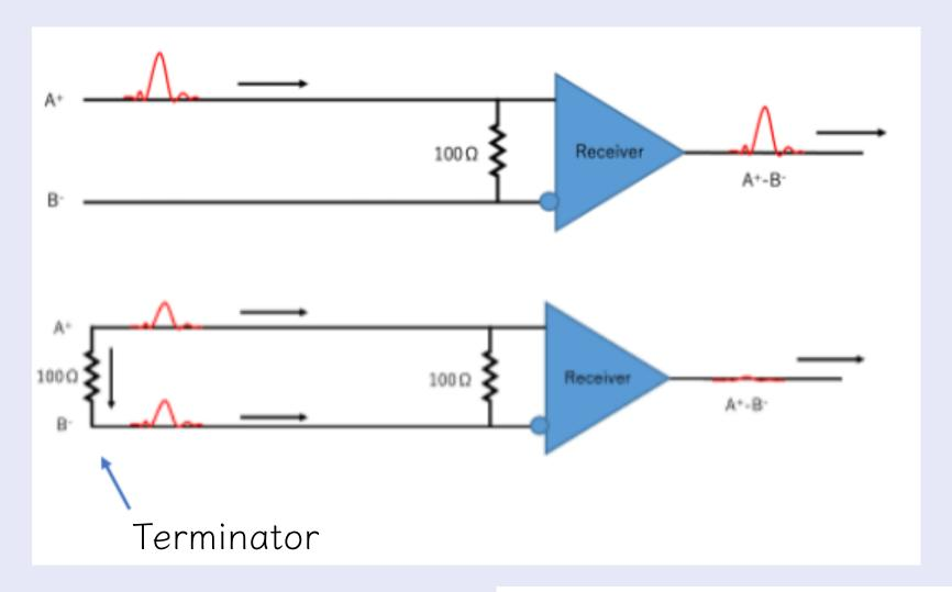
By attaching a terminator at the open end, we intend to common-mode the noise and cancel it out.
