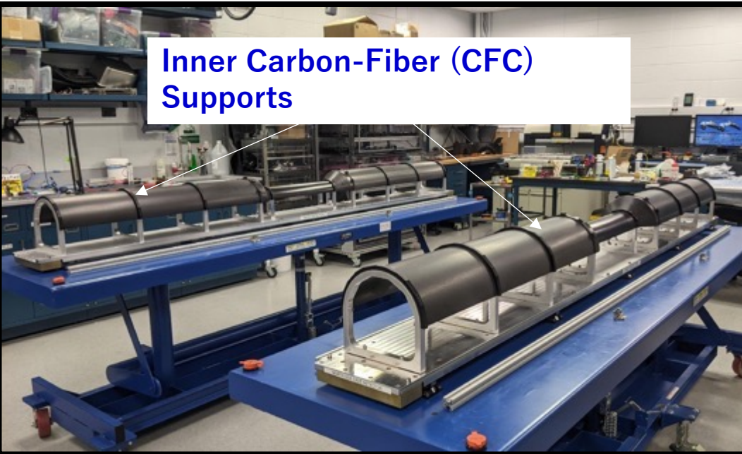
Silicon Strip Layers Mounted on CFC Support
