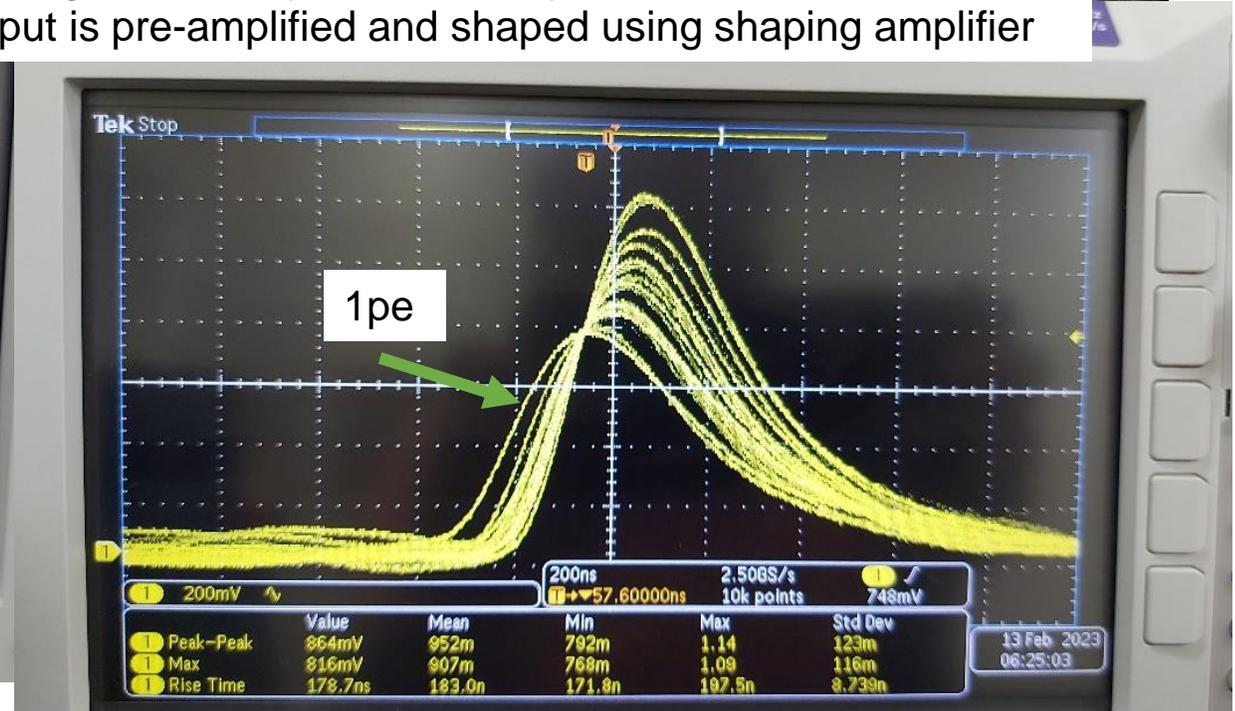
Single photo e- pulses and after-pulses are visible
