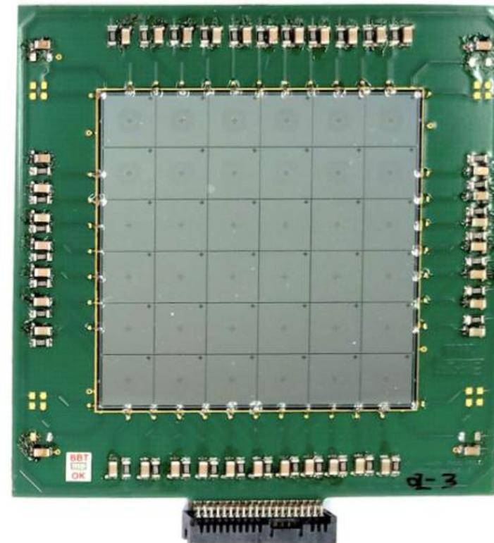
Design of 6x6 n-type detector developed by BEL, Bangalore
