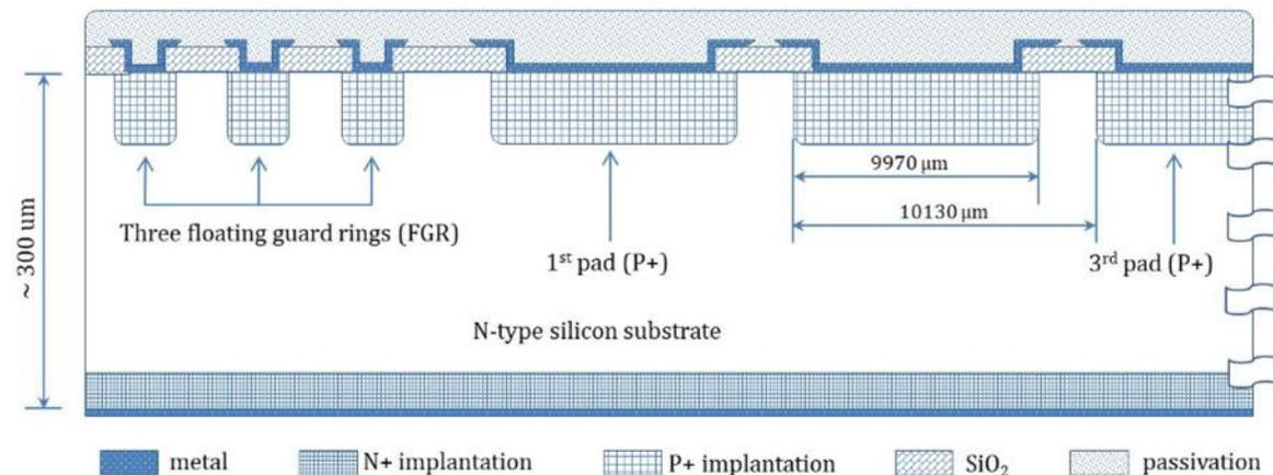
**Figure 2.** Cross-section of the silicon pad sensor: three pads with the peripheral region (Distances are not to scale).
