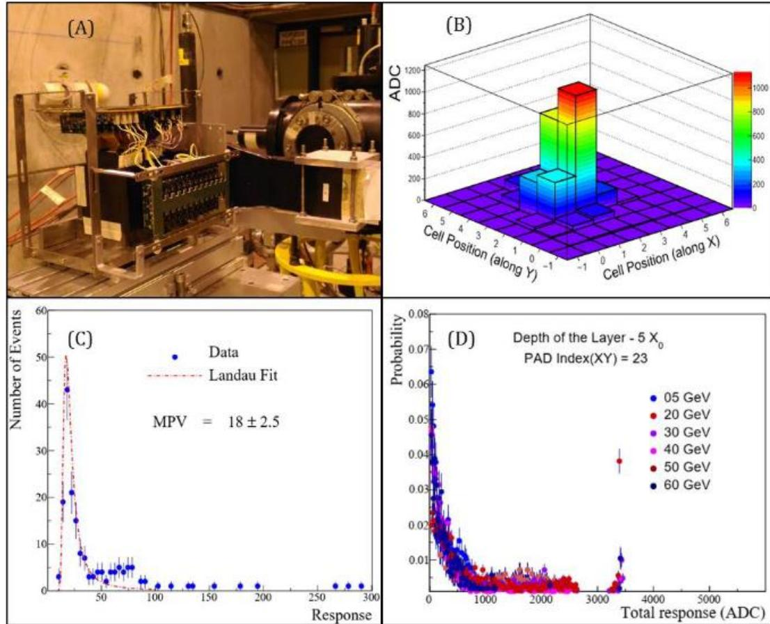
**Figure 11.** (A) Experimental setup at SPS-CERN. (B) 3-D plot showing the energy deposition in terms of ADC count for different pads in a particular sensor layer (layer eight among the 19 layers) in response to a 30 GeV electron beam. (C) The typical response of a pad in a particular sensor layer to a 120 GeV pion beam (MIP) [15]. (D) Response of pad 23 (array coordinate 2,3) of the sensor situated in the 8th layer for a wide range of incident energies of the incoming electron beam.
