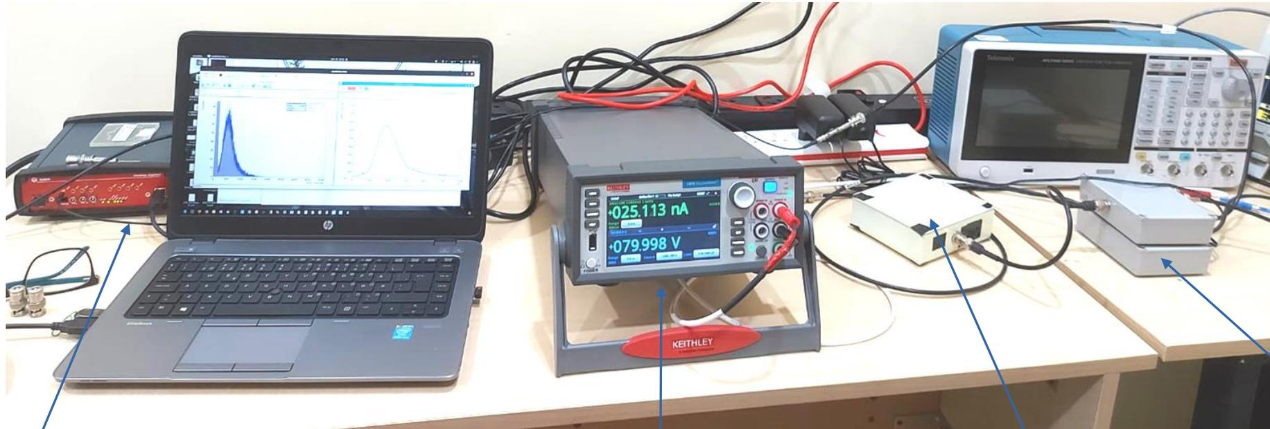
CAEN Digitizer (DT5730) 8 ch, 14 bit resolution, 500 MS/s sampling rate, 2Vpp dynamic range
