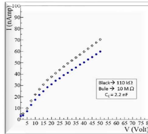
Radiation damage study was done at VECC-K130 cyclotron. The data are being analyzed. The dose, irradiate did not damaged the response in terms of I-V. Next experiment with higher dose is planned.
