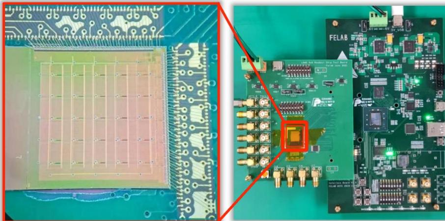
channels with a common source preamp integrated
