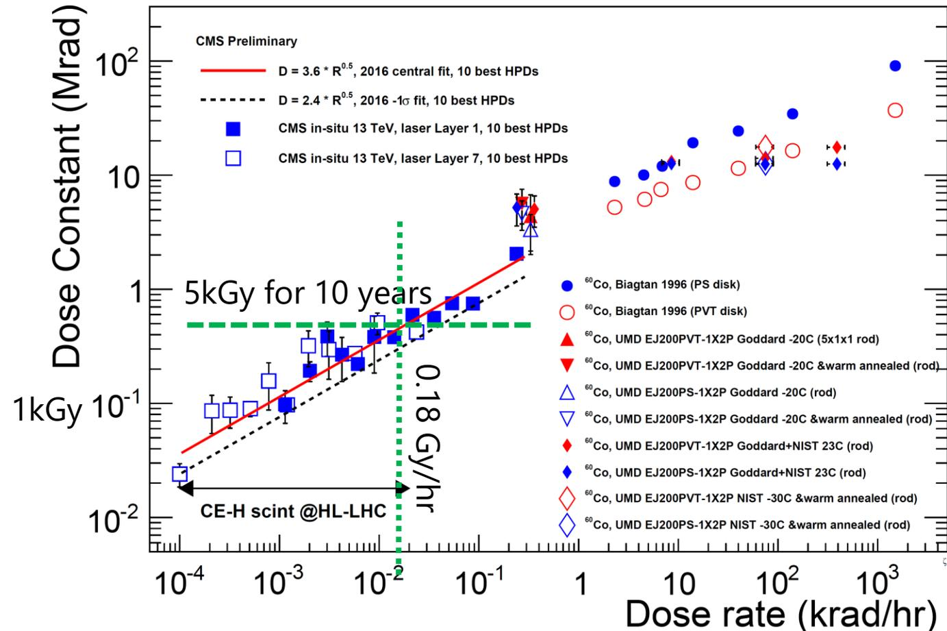
Figure 2.10: Dose constant,  $D_c$ , versus dose rate,  $R$ , for both in situ measurements from CMS (boxes) and dedicated studies. Lines corresponding to  $D_c = 3.6 \times R^{0.5}$ , and  $D_c = 2.4 \times R^{0.5}$  are shown. The in situ measurements refer to SCSN81, a PS based scintillator used in the endcaps of the present detector.
