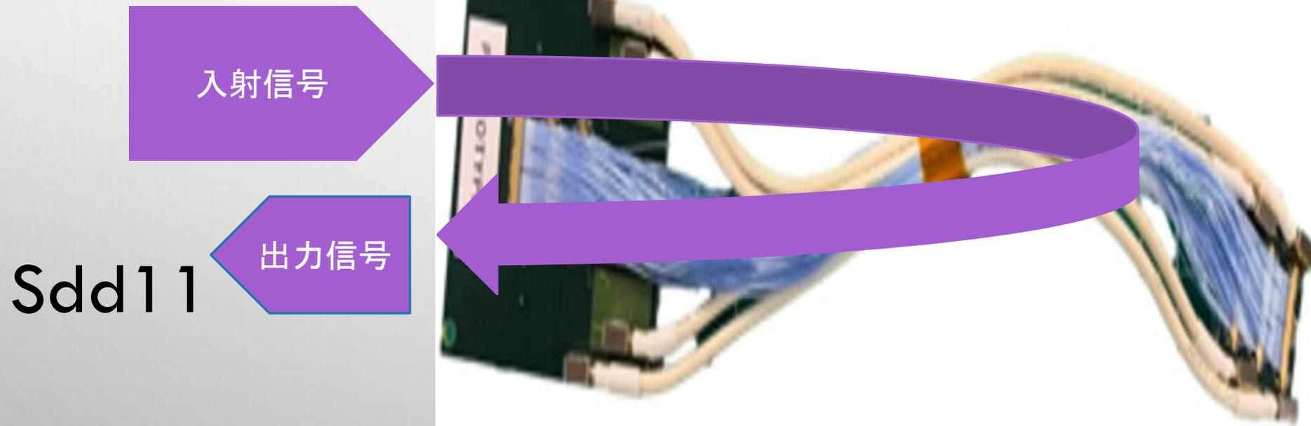
$$S\text{パラ} = \frac{\text{出力信号}}{\text{入射信号}} = \text{反射損失}$$
