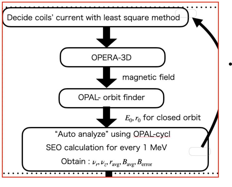
Useful data like  $B_{avg}$ ,  $r_{avg}$ ,  $F^2$ ,  $B_{error}$  can be obtained.
