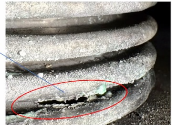
Feedthrough bellows rupture
