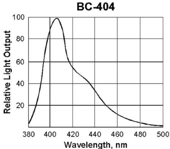
(a) Emission spectrum of the BC-404 scintillator. The peak of the emitted wavelength is at 408 nm.
