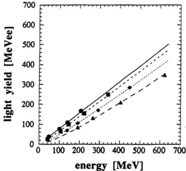
Figure 1: Light output (in electron-equivalent energy) of BaF<sub>2</sub> scintillator for protons (circles), α-particles (squares), <sup>7</sup>Li (diamonds) and <sup>9</sup>Be (triangles). The data are of Ref.[7] while the lines result from the integration of Birk's law (Eq.1).
