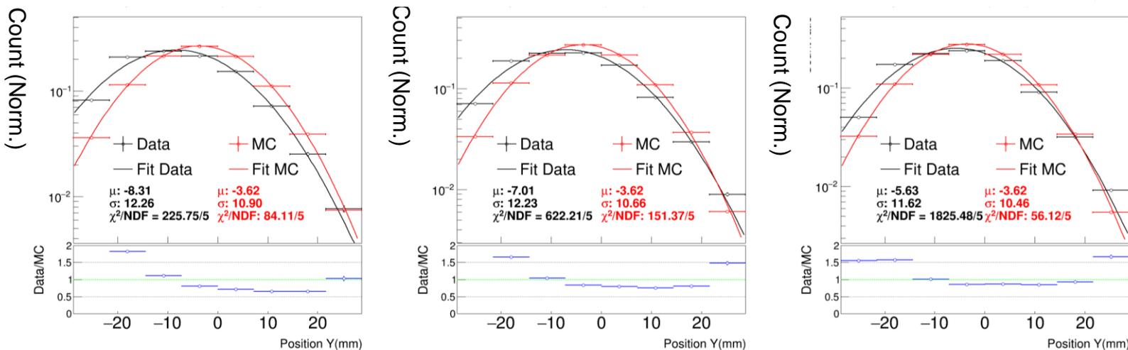
Data have wider beam profile than MC. MC will be further fine tuned.
