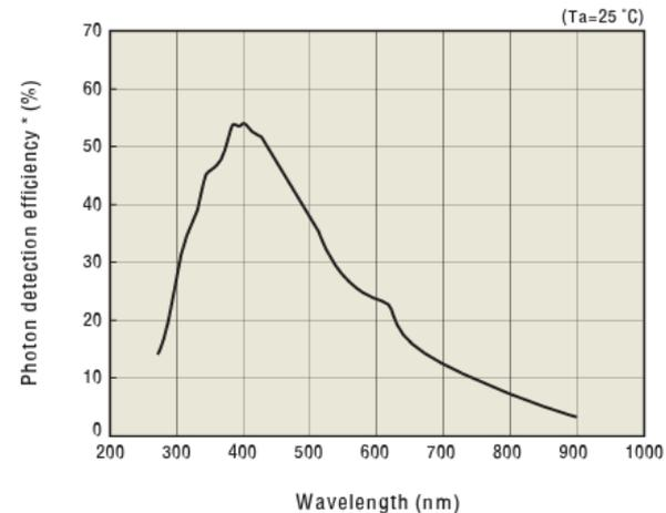
(b) Absorption spectrum of the SiPM. Peak sensitivity wavelength is at 400 nm.
