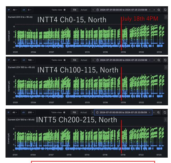
The drawing currents have been slowly increasing and the slope may get a bit steeper around July 18th.
