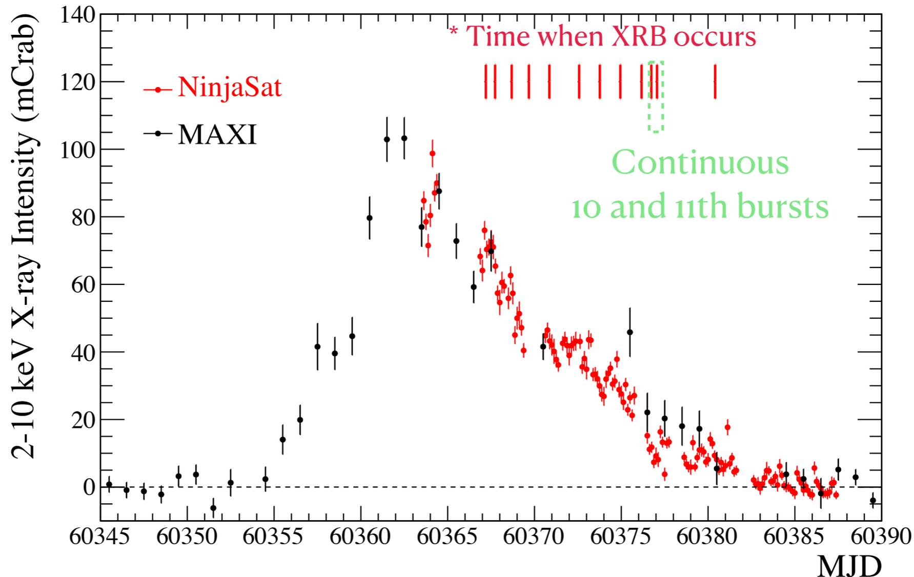
**Fig. 1.** 2–10 keV light curves of SRGA J1444 monitored by NinjaSat (red) and MAXI (black) with the binsizes of 3.0 hr and 24 hr, respectively.
