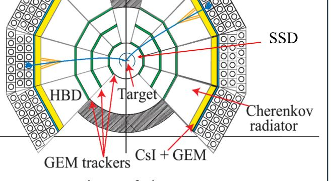
Cross section of the spectrometer
