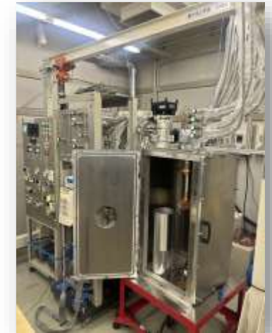
Test chamber and the gas handler at Konan University
