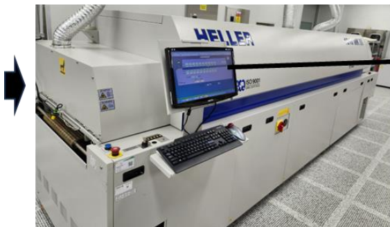
4) Solder reflow process for bump solidification
