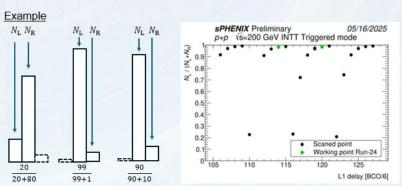
INTT have been operated in optimized delay settings, with ~99% hits correctly recorded within a single BCO!
