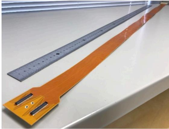
**Figure 16:** A photograph of the 1.11 meter long BEX cable.
