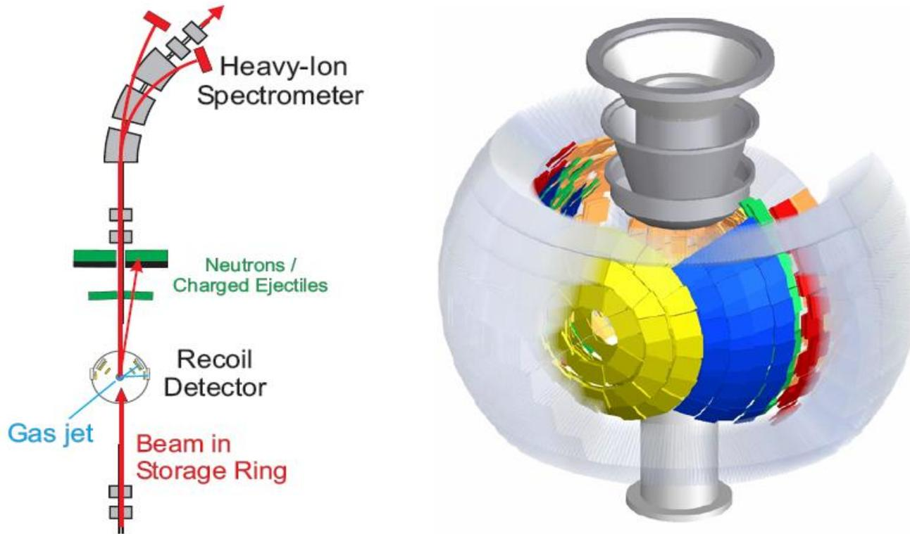
**Figure 1:** Schematic view of the EXL detection systems. Left: Set-up built into the NESR storage ring. Right: Target-recoil detector surrounding the gas-jet target.
